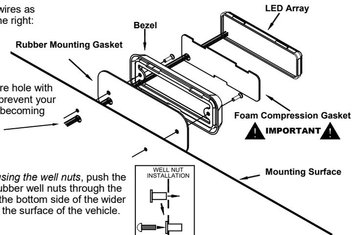
4. Seal the wire hole with silicone to prevent your wires from becoming damaged.
